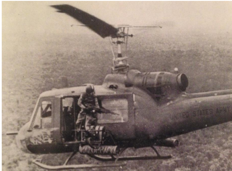
Figure 4. An armed Huey used in Vietnam equipped with an M-60 machine gun mount and seven-round rocket pods.
